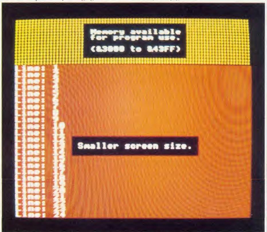
This standard model 20k screen shows the area used for the shrunken screen (at the bottom) and the area liberated for use by Basic programs (at the top)
